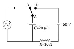
(A) Magnitude of the maximum charge on the capacitor before  $t = \frac{7\pi}{6\omega}$  is  $1 \times 10^{-3}C$ . (B) The current in the left part of the circuit just before  $t = \frac{7\pi}{6\omega}$  is clockwise.
